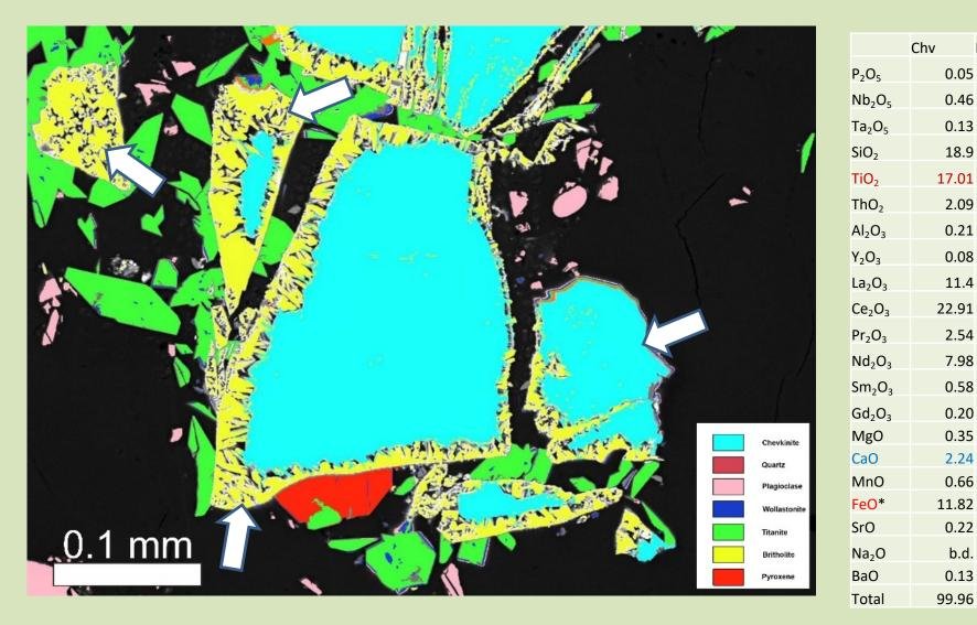
Note characteristic, for coupled dissolution and precipitation process (similar to the examples presented by Ruiz-Agudo et al. (2014), position of britholite crystals (it outlines the original shape of the chevkinite crystals)
