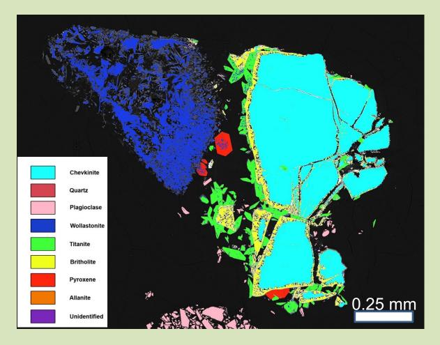
Wollastonite is unusual in natural occurrances of chevkinite hydrothermal alterations but in the experiment it may reflect excess of Ca in the fluid after formation of titanite and pyroxene.
